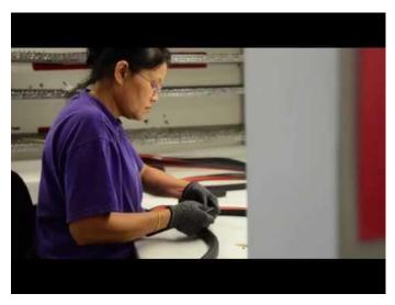
After cutting, cold-bonded gaskets are assembled by skilled production personnel.
